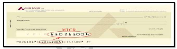
MICR is also an input device is commonly used in banks because of a large number of cheques to be processed. The bank's code number and cheque number are printed on the cheques with a special type of ink that contains particles of magnetic material that are machine readable. This reading process is called Magnetic Ink Character Recognition (MICR).
