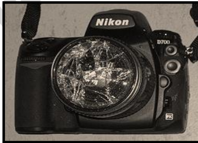
Nikon D700 with broken filter B+W UV 010 and lens Nikkor 28-85mm
